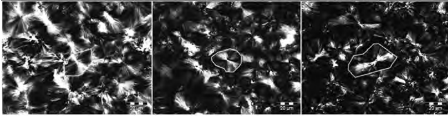
Figure 10. ~ Polarized light micrographs of thin sections of polypropylene with compatibilizer, produced with different mold temperatures (left 15°C, middle 40°C, right 70°C).
