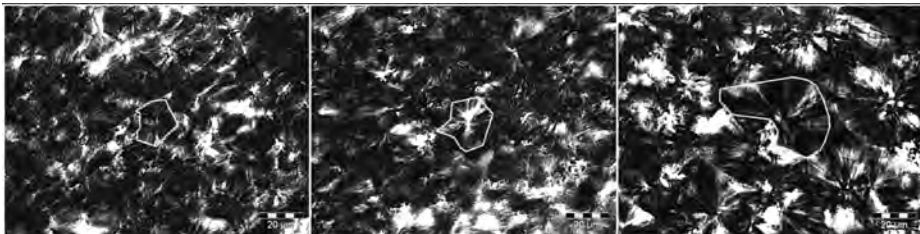
Figure 12. ~ Polarized light micrographs of thin sections of WPC containing 10 wt% of wood, produced with different mold temperatures (left 15°C, middle 40°C, right 70°C).
