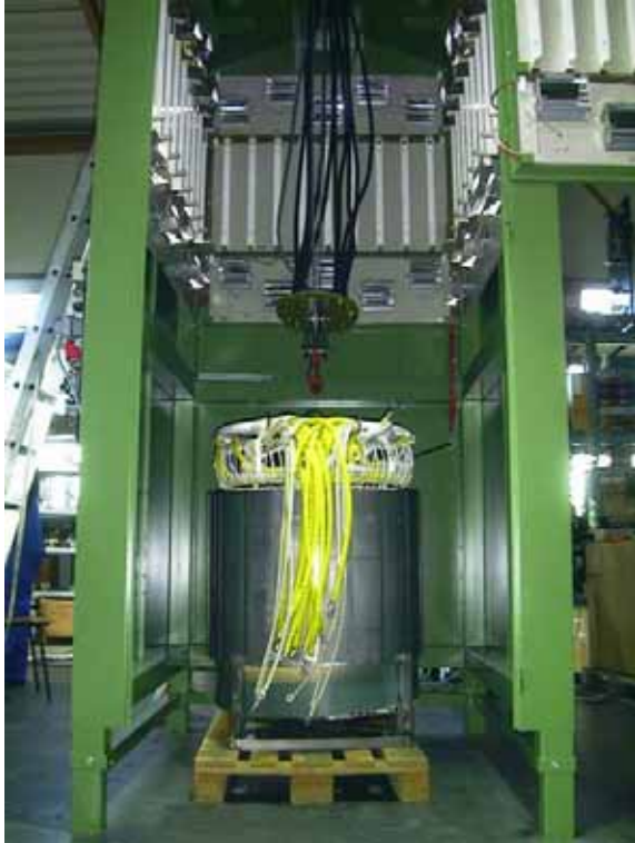
Figure 1: Pilot plant of company Gottlob Thumm in Germany. A stator of a wind power generator is prepared for impregnation.
